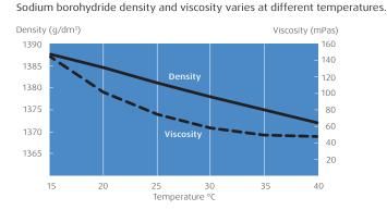
We also prepare sodium borohydride solutions for customers' special needs, for example Hydrifin C concentrate containing 20 % NaBH<sub>4</sub> and 20 % NaOH, balance water.
